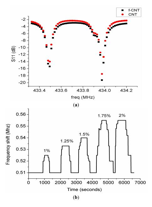
Figure 10. (a) Response of CNT and functionalized CNT to hydrogen gas; (b) Plot of frequency shift *versus* time for different hydrogen gas concentrations.
