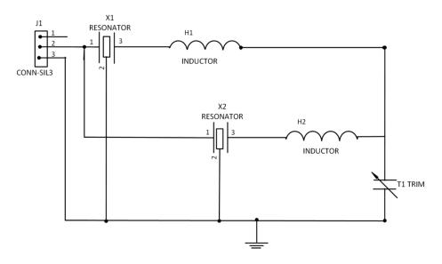
Figure 1. Schematic of DSAWR circuitry.
