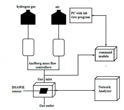
Figure 5. Gas sensing measurement set-up schematic.
