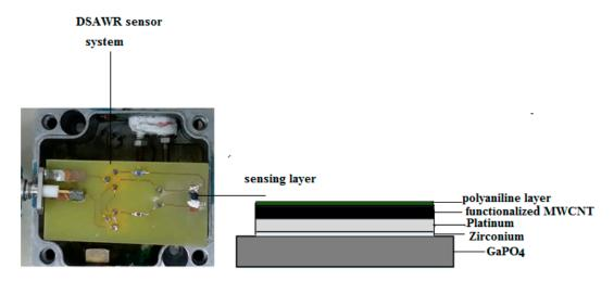
**Figure 4.** (a) Fabricated DSAWR sensor with the sensing layer integrated into the system placed in a test cell; (b) Side view of the sensing layer (thickness not to scale).
